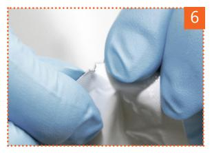
Tear the aluminium envelope open at the notch. Once the device has been taken out of the envelope its stability is of short duration, especially in a humid environment.
